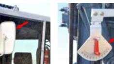
Guide swing angle indicator by pendulum
