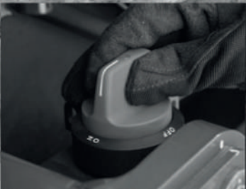
Battery cut-off switch
